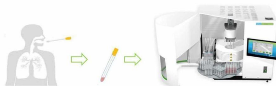
Figure 1 Automated RNA extraction workflow: in a fume hood the dry swabs need to be equilibrated in a physiological/isotonic solution (e.g. PBS) followed by a short incubation. From this liquid 300 \mu L is transferred as sample into a deep-well-plate followed by the addition of 4 \mu L Poly(A) buffer, 10 \mu L Proteinase K and then 300 \mu L Lysis buffer before starting the automated extraction.
